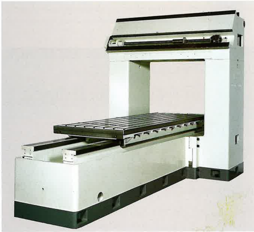
Highly rigid bridge type construction
