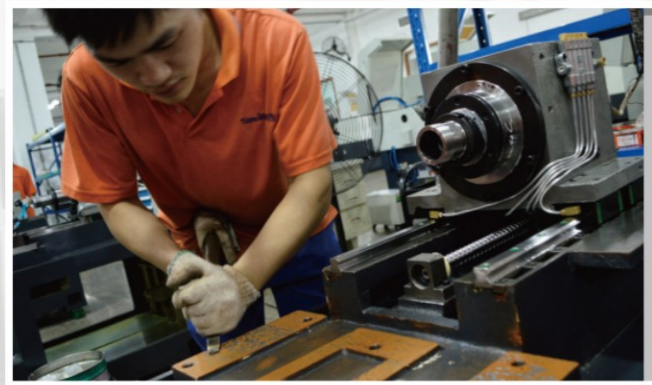
The scraper of main mounting surface
