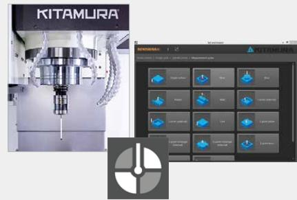
**Set and Inspect** on-machine probing app makes probing easy and is standard on the Arumatik®-Mi Pro CNC. An intuitive interface guides you through the process of creating a probe cycle and automatically generates the required machine code, loading it to the Arumatik®-Mi Pro. No probing experience or machine code knowledge required!
