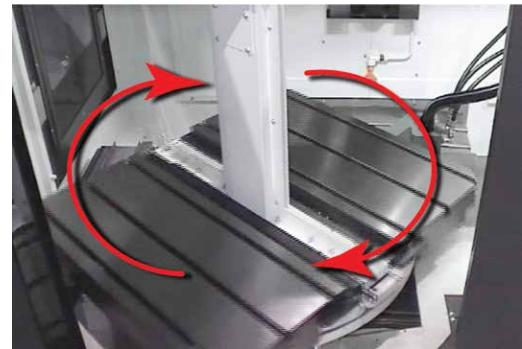
Easily load and unload parts when the machine is in cycle with a high-speed, factory installed 2-station 180-degree rotating automatic pallet changer.
