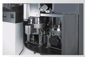
• Automatic turning head exchange
