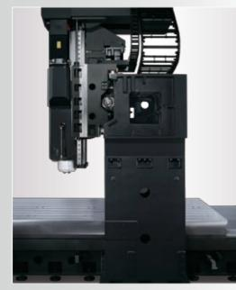
Cross section shown the cross beam designed for higher rigidity with 20% enhance above.
