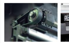
Torque limit mechanism on X/Y/Z axes.
