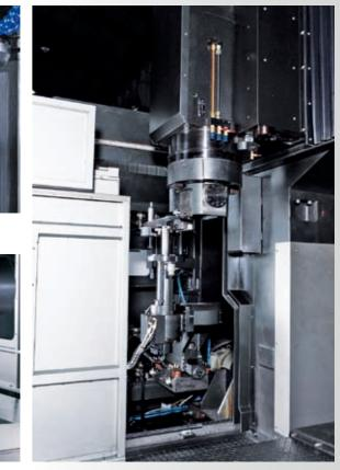
• Automatic turning tool exchange.
