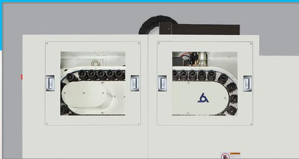
*The high-performance ATC holds **40 tools** and provides "operator-friendly" accessibility for easy tool loading.*
