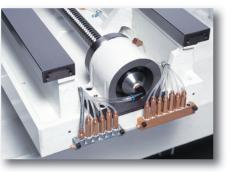
Ballscrew temperature is precisely controlled by an internal ballscrew cooling system. This eliminates thermal growth and promotes rigidity assuring peak machining precision even under prolonged heavy cutting conditions.
