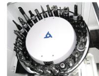
Tool Handling Efficient tool handling slashes idle time to maximize machining profit. The Mycenter-3020G ATC uses a memory-random tool selection system for smooth idle-free tool changes. Its generous 30 tool ATC enhances machining capability.
