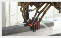
Induction hardened solid box guideways with linear scale feedback on all axes with twin ballscrew design in X,Y & Z axes.
