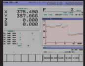
Intelligent Advanced Control System. Controls the effects of heat displacement in order to ensure continuous accuracy in machining. Minimizes head displacement to less than +/-5 microns. 6 sensors positioned on the machine measure and monitor temperature of machine and compensation guarantees positioning accuracy of +/-0.002mm (+/-0.000079") / Full stroke. Kitamura patented system since 1998.
