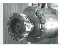
*With Power to handle the toughest cutting conditions* the Mycenter-HX630G features a 53HP, high-torque, 4-step gear driven spindle that delivers high-efficiency cutting performance with low energy consumption. 8,000min<sup>-1</sup> and 12,000min<sup>-1</sup> configurations are available.
