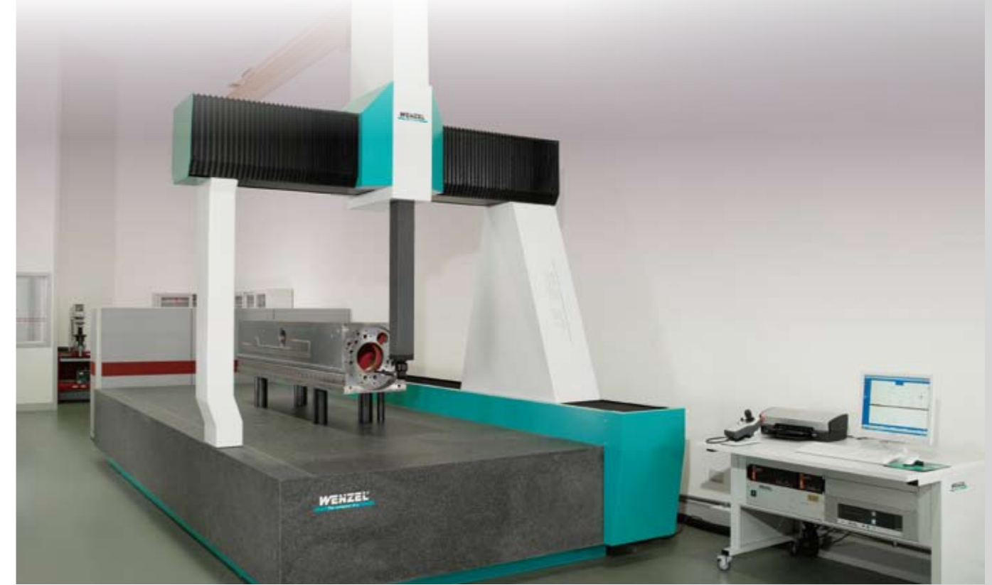
Every key components quality assurance was by German WENZEL3D CMM machine.
