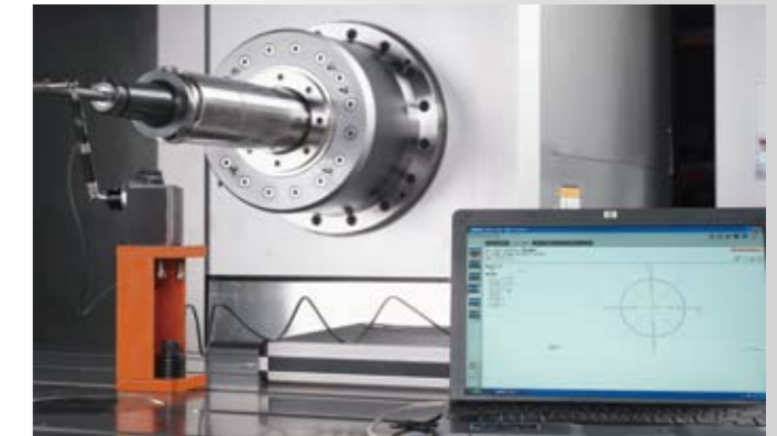
Ball bar Circular interpolation measurement.
