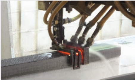
Induction hardened solid box guideways with linear scale feedback on all axes with twin ballscrew design in X, Y & Z axes.
