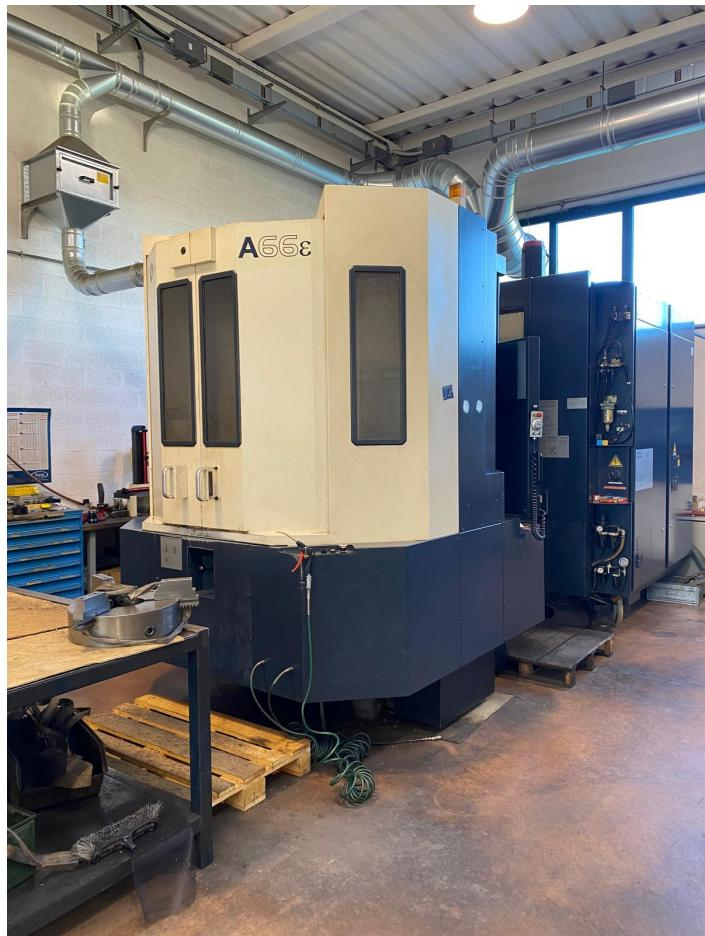
**Type:** Horizontal machining center Pallet changer
